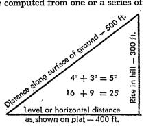
hypotenuse. Thus, if a hillside rises 300 feet in a distance of 500 feet, as measured along the ground, the horizontal or survey distance shown on the plat should be 400 feet, not 500 feet.
