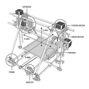
Fig. 1 – A "Cartesian robot" style 3D printer. 30
